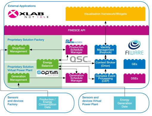
The Generation Schedule Manager DSE provides information about the VPP's energy generation. The Production Schedule Manager DSE provides the 3 production plans based on the energy requirement. The Energy Balancer takes the output of these 2 DSEs to plan how to balance the energy production and consumption. Data to identify deviations from the plan during the production is sent to the Complex Event Processing GE.
