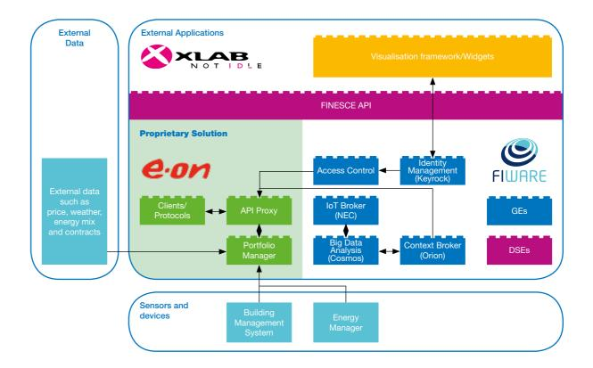
The **API Proxy** provides the external trial API and acts as a frontend integrator towards FI-Lab. As for the executing of Big Data related use cases, the **Context Broker GE (Orion)** has a very central position and interfaces to **Big Data Analysis (Cosmos). Identity Management (Keyrock)** is used for a single-sign-on to the external Visualization framework/Widgets.
