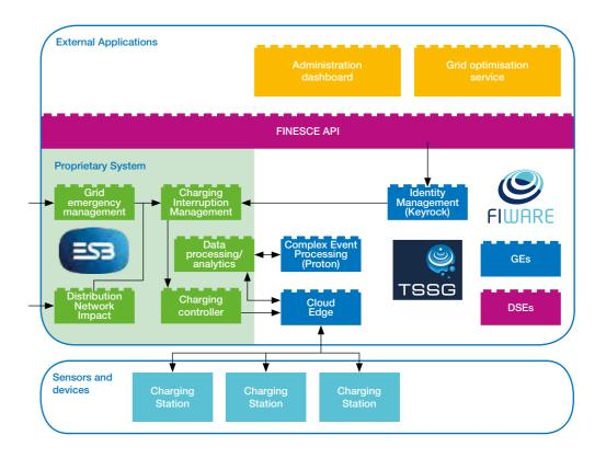
The **Distribution Impact**, provided by an external DSO system authorises the EV charging based on its knowledge of the effect that a given EV charging schedule has on the LV and MV grid conditions;
