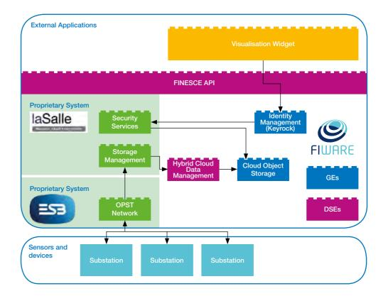
**Hybrid Cloud Data Management DSE** contains the parts of the Storage System which provide access to the local and distributed storage. The API for controlling the DSE is offered as part of the FINESCE API.
