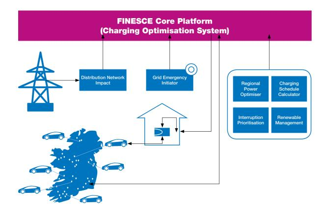
The heart of the charging optimization contains all data collected during the trial as well as configuration data to be taken into account by the charging optimisation algorithm. The management and control software of the Electric Vehicle Supply Equipment are being developed and hosted by WIT. Additionally an API is provided allowing access to trial data for internal partners and also SMEs or other third parties that want to use these data.
