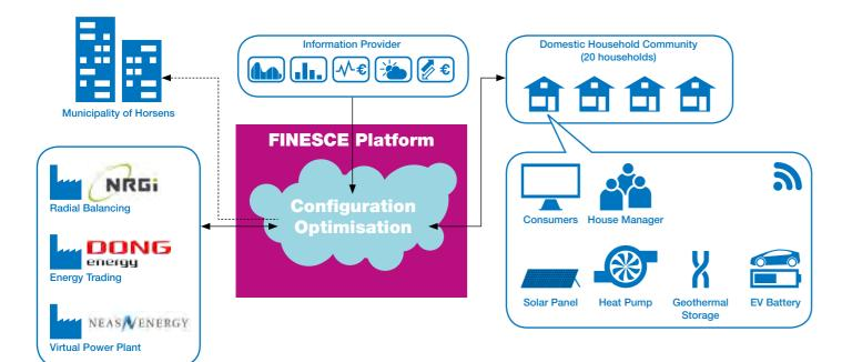
The families have access to real-time information about energy consumption. This happens via an intelligent IT cloud system, through which utility companies, energy and equipment suppliers and other third parties can also interact with the different houses. The new equiment, combined with the presentation of useful information positively influenced the families' behaviour and energy consumption.
